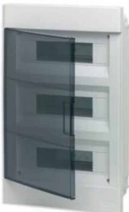
V52436 36 modules, delivered with DIN rail (60715 TH35), RAL 9003 white, with transparent door, fumé. Dissipated power: 68 W
