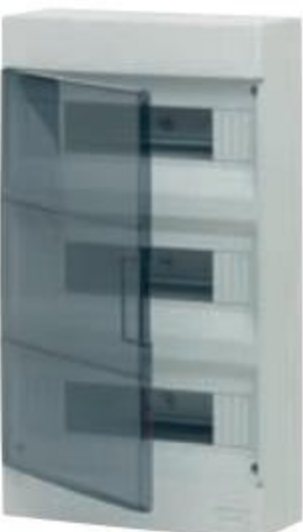
V50436 36 modules, top and bottom knockouts, with DIN rail (60715 TH35), RAL 7035 grey, with transparent door, fumé. Dissipated power: 37 W
