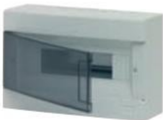
V50412 12 (12+1) modules, top and bottom knockouts, with DIN rail (60715 TH35), RAL 7035 grey, with transparent door, fumé. Dissipated power: 18 W
