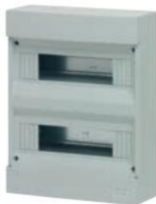
V50324 24 modules, undrilled walls, with DIN rail (60715 TH35), RAL 7035 grey. Dissipated power: 37 W
