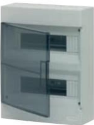
V50424 24 modules, top and bottom knockouts, with DIN rail (60715 TH35), RAL 7035 grey, with transparent door, fumé. Dissipated power: 31 W
