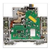
Combined design with electronic differential protection module, class D varistor and built-in circuit breaker of VA47-60 series provides for 4 types of protection: against differential (leakage) current; short circuit; overload; and protection of device internal components against pulse surges.
