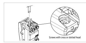
The terminals, located in the rear part of the devices, are manoeuvrable even after coupling the component to the support, and are suitable for both flexible and rigid cables. The components are supplied with the screws of the terminals open, to reduce wiring times.
