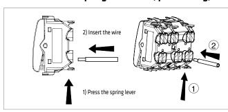
The spring terminals allow you to carry out the wiring in a shorter time, and without using screwdrivers or other tools. To insert the cable, it is necessary to press the orange lever (opening of terminal). Releasing the lever, the terminal closes automatically, firmly blocking the cable.
