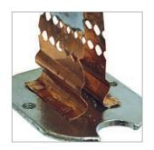
Fuse element is made of phosphorous bronze (orichalcum with addition of phosphor) and securely fixed by means of spot welding with fuse terminals.
