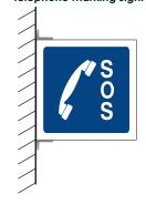
Single sided luminaire mounted parallel to the wall with marking distances from the escape routes.
