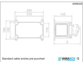
Top: 1xM12, 1xM20, 2xM25 or 2xM32 Bottom: 1xM12, 1xM20, 2xM25 or 2xM32
