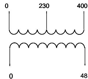
**Single phase insulating transformers****Primary voltage 230, 400V. Secondary voltage 0-110V. Thermal class B. DIN rail**
