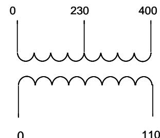
**Single phase insulating transformers****Primary voltage 230, 400V. Secondary voltage 0-230V. Thermal class B. DIN rail**
