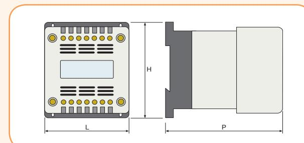
**Single phase safety transformers****Primary voltage 230, 400V. Secondary voltage 0-24V. Thermal class B. DIN rail**
