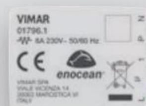
1-relay actuator with EnOcean module
