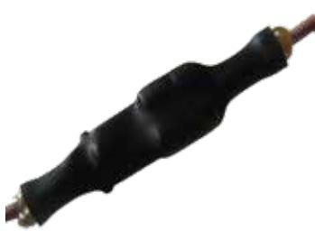
Manufactured by co-extrusion of polyolefin and hot-melt adhesive. Suitable for electronics and automotive industry where components are of irregular sizes, shapes and protection against water and moisture are important. Provides both insulation and sealing for protected articles.
