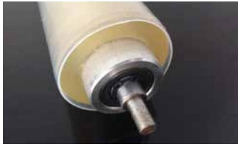
Our PTFE sleeves are applied to a variety of rolls and tubes guaranteeing the unique properties provided by Shrinktech. We supply you the perfect quality for your requested diameter! The application of the sleeves is a simple process: the sleeve is slipped over the roller and heated with a hot air gun, which allows the sleeve to shrink to a tight fit on the roll.
