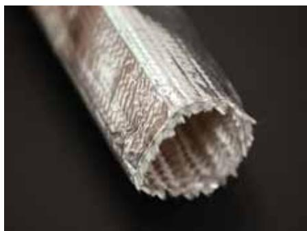
STF-ALU is a flexible sleeve made of fiberglass braid covered with an aluminum foil. The tube offers a continuous working temperature of -40°C up to +200°C. Its smooth and reflective outer surface provides a very reflective barrier to radiant heat. Used within the automotive sector.
