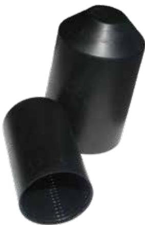
Recommended for use both in open air and on underground power distribution cables with PVC, lead or XLPE sheets. Definitive recovery with the layer of spiral coated hot melt adhesive. Protects power cables up to 1 kV and telecommunication cables. Resistant to oxydation, ozone, UV radiation.
