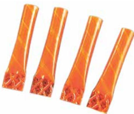
Multilayered precision wound protective end cap made from DuPont™ Kapton® film and Nomex®. Designed for use in varnish impregnated electrical motors, LKTC end caps maintain electrical resistivity, dimensional stability and strength at high temperatures and in the most demanding applications. Sonic welded seal is chemically resilient and further contributes to the robustness and reliability of the eventual product.
