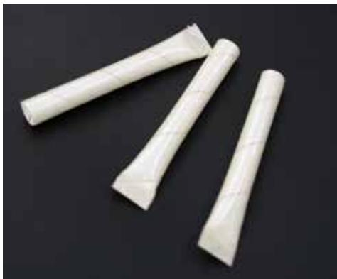
LARC heat shrink caps prevents line failures in hermetic motors by securing and insulating electrical connections. Shrink-on tting both prevents the dispersal of debris withing a motor and provides comprehensive mechanical and electrical protection, cutting line failures arising from vulnerable connections.
