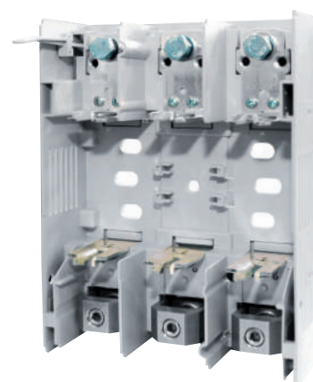
RBK 1 pro VD-M for installation on mounting plate, picture of fuse switch disconnectors without fuse links cover and terminal shrouds, top cable terminal - M screws, bottom cable terminal - V-clamps, (RBK 1 pro VG-M - bottom cable terminal - M screws, top cable terminal - V-clamps)
